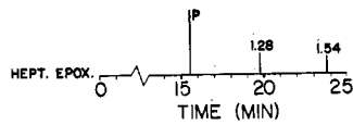
Figure 4. Uv degradation pattern of heptachlor epoxide. Separation carried out on a column packed with 5% OV-225 on 70/80 mesh Anakrom ABS
